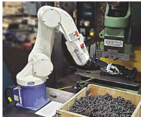
World's first entangled part, bin-packing robot used in the spring and wire form manufacturing operation at India Springs Inc.
