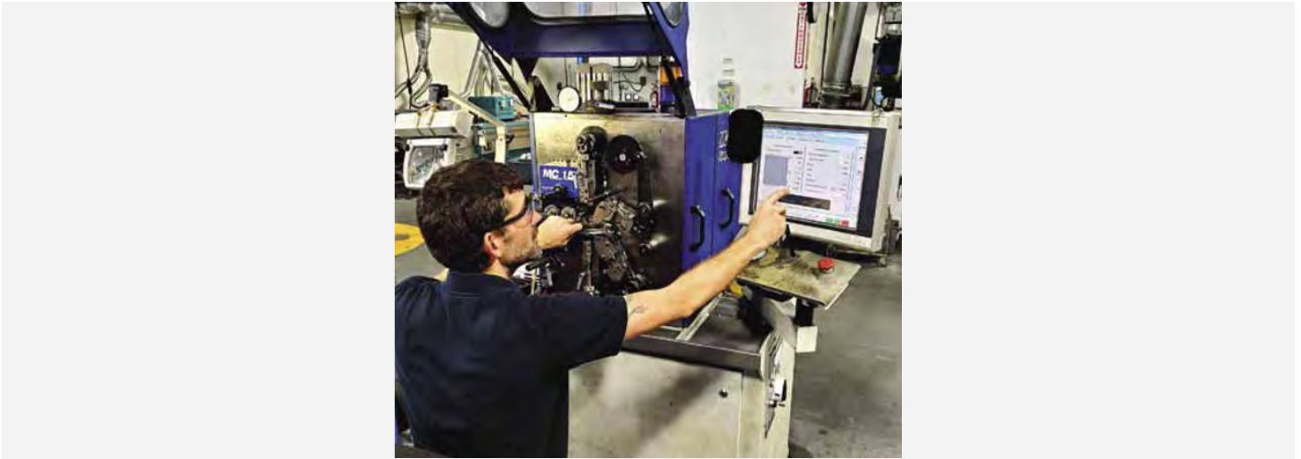
A Southern Spring and Stamping team member programs its Simplex spring coiler machine. Photo courtesy of Southern Spring and Stamping.
