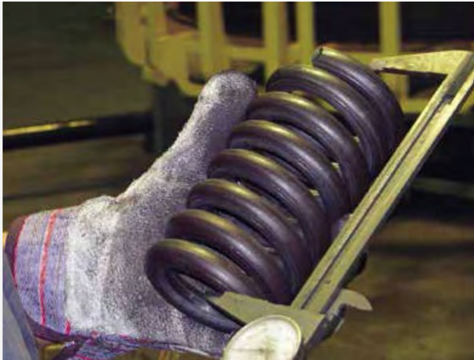
One of Ace's coilers measures a spring to verify that its height matches the specifications. Photo courtesy of India Springs Inc..
